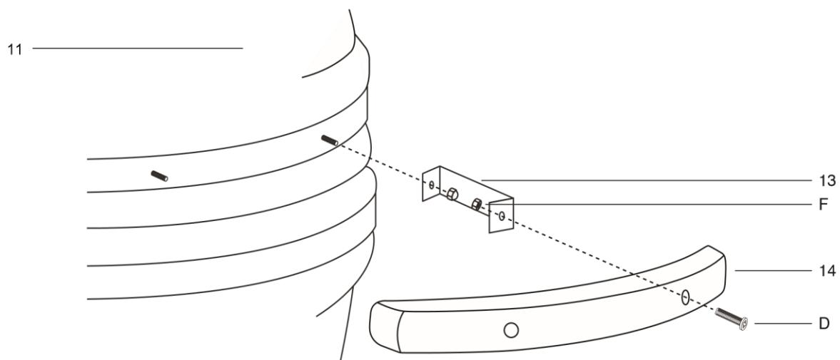
**STEP 12** - To attach the handle (14) to the lid of the Kamado Grill (11) start by attaching 2x handle brackets (13) using the 2x pre-attached bolts and dome headed nuts. Attach the handle (14) to the brackets (13) using 2x bolts (D) and nuts (F)
