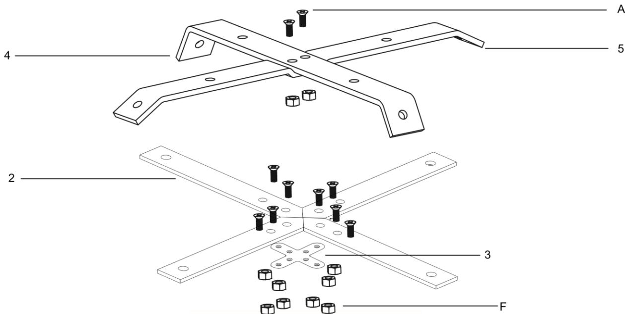
Position the parts on a flat surface that will not scratch the finish of the nest components, paying close attention to the joint overlap in illustration the 2pcs Upper cross brace(4&5) and 2pcs Lorer cross brace(2).
