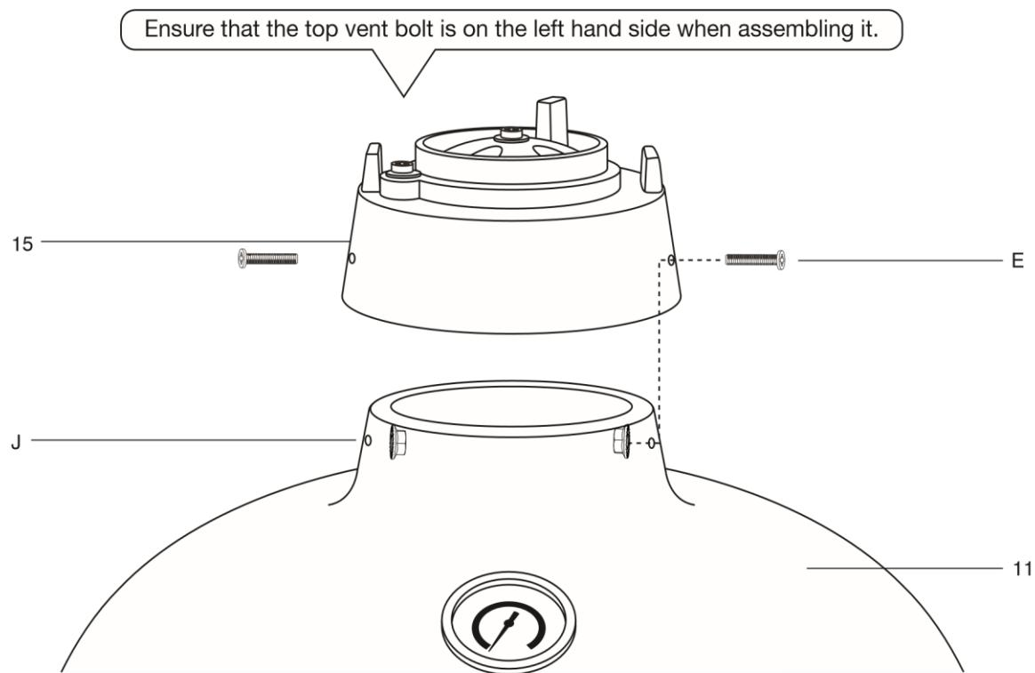
**STEP 13** - To attach the top vent (15) to the Kamado Grill (11) place it on top and align both the bolt holes. Secure using 2x bolts (E) and nuts (J). Ensure that the top vent bolt is on the left hand side when assembling it.
