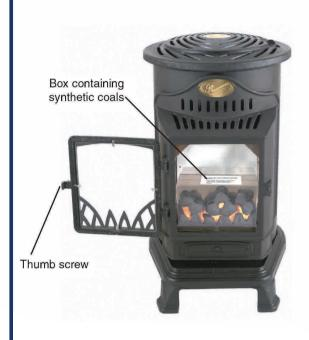
Open the heater door by loosening the thumb screw. Remove the box containing synthetic coals from the heater. Carefully remove the synthetic coals from the box.
