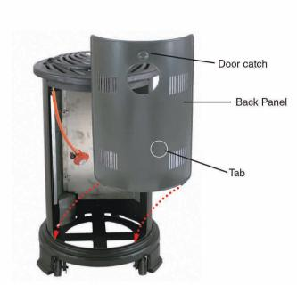
Fit the back panel of the heater by positioning the tabs on the bottom of the door into the inside of the rim at the bottom of the heater. Then push the panel flush with the back of the heater and turn the door catch to the up position to secure the panel.
